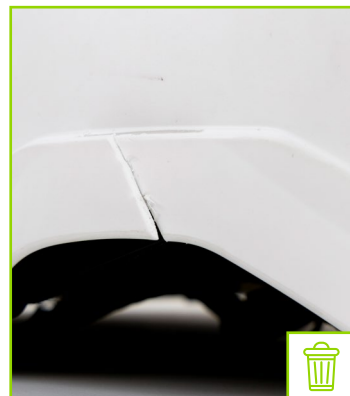
Cracked accessory slot
