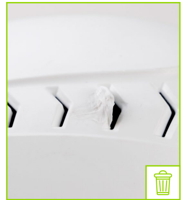
Shell with deformed ventilation hole
