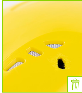
Perforated external shell
