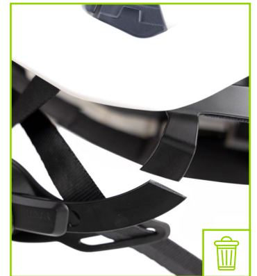
Broken regulation system branch
