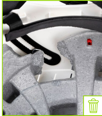
Inner shell missing part
