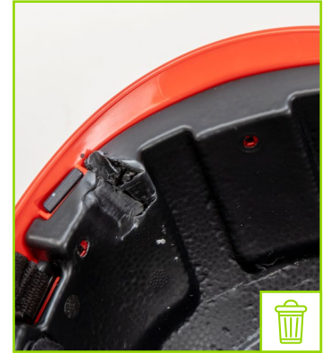
Deformed inner shell
