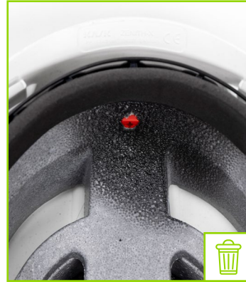
Inner shell with flame burn marks
