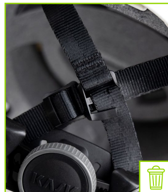
Broken rear adjustment buckle
