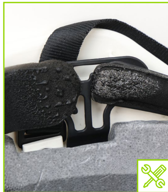
Liner with flame burn marks
