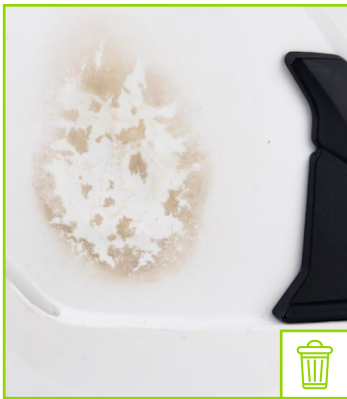
External shell with traces of chemical substance
