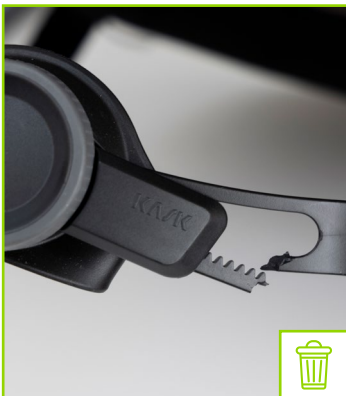
Broken adjustment system branch
